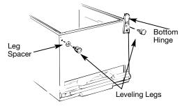
**6.** Remove the leveling leg below the bottom hinge and the leveling leg and leg spacer at the opposite corner.
